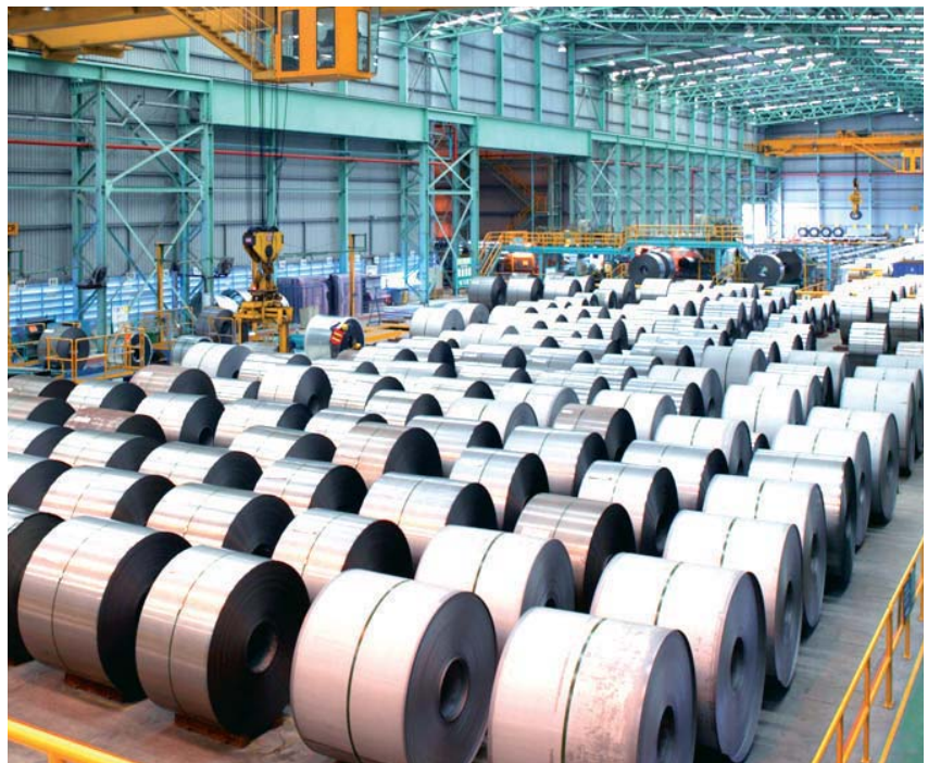
The special coating on the sheet is composed of 55% aluminum and 43.5% zinc with 1.5% silicon. The significance of this material is that its corrosion resistance is vastly superior to tradition products such as galvanized steel, yet it costs no more.
