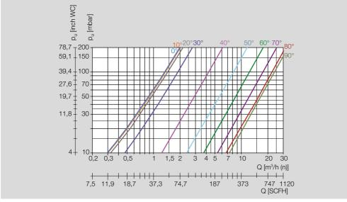
The characteristic flow rate curves have been measured with the valve closed.
