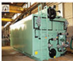
Cleaver Brooks Water Tube Boiler
