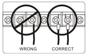
Fig. 2-1: Wiring the sub base terminals
