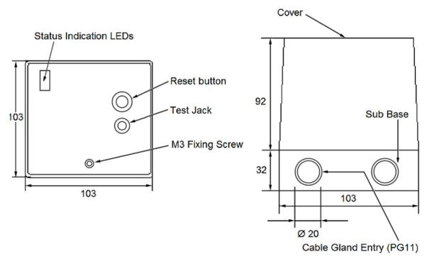
Fig. 1: External Dimensions (in mm)
