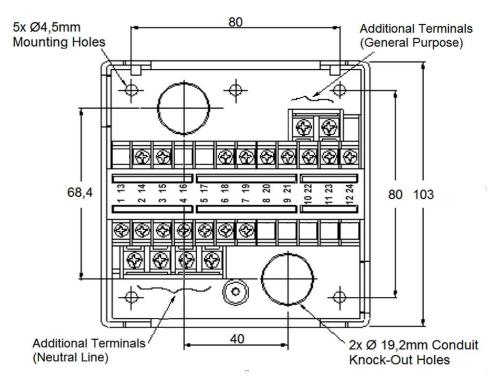
Fig. 2: Mounting dimensions of sub-base and terminal layout
