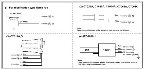
Fig. 4-1: Wiring a flame detector
