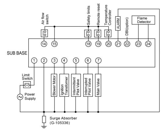
Fig. 3-1: Example of wiring to external equipment (see fig 3-2 for more)
