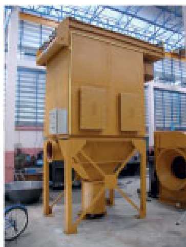
Dust Collector or Bag Filter
