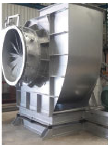
Blower + Inlet Damper
