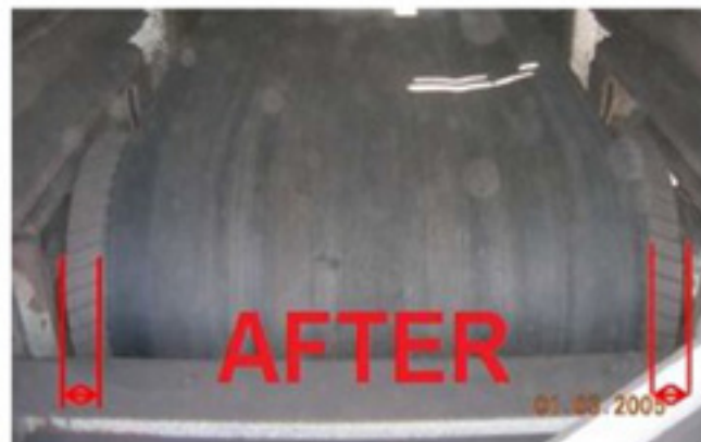
Before After install Tru-Trac at tail pulley
