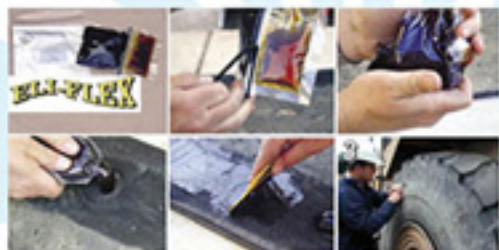
ELI-FLEX polyurethane resin quick and easy repairs for damaged conveyor belting and tier.
