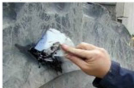
Repair for rip of truck tire
