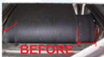
For tracking the belt conveyor miss alignment to run in the center
